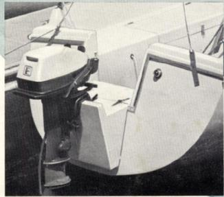
Fold down transom section forms strong outboard motor bracket with no extra pieces to stow.
