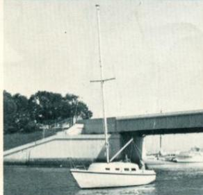
Mast in position to raise with heavy cast hinge already pinned, gooseneck attached to heel track and steady wires fastened.
