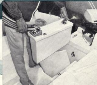
Scabbard type removable inboard rudder "plugs in" to well providing solid action rudder post.
