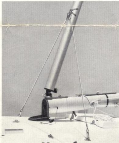
Backstay hardware with quick release pin and simple backstay tackle which eliminates the need for resetting turnbuckle adjustment each time mast is set.
